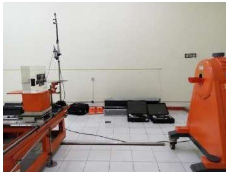
FIGURE 2. Exposing TLD against gamma source ^{137}\text{Cs} of OB 85
