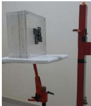
FIGURE 1. Exposing TLD against beta source ( ^{90}\text{Sr} , ^{85}\text{Kr} , and ^{147}\text{Pm} ) with using BSS 1
