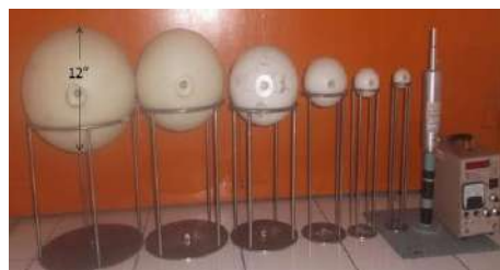
FIGURE 2. Bonner sphere spectrometer at Neutron Laboratory of National Nuclear Energy Agency (NNEA)
